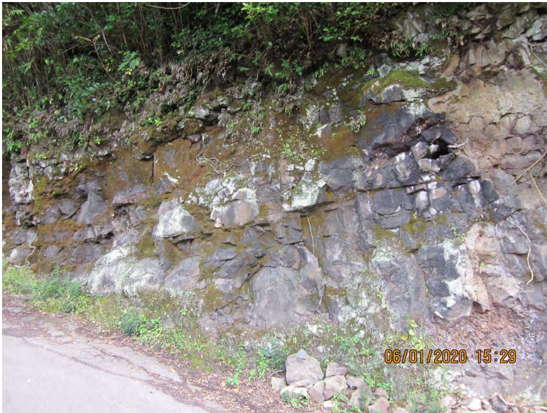
Photo 7. Transect F-W-04, Central Section. Jointed Basalt Outcrop with Residual.
