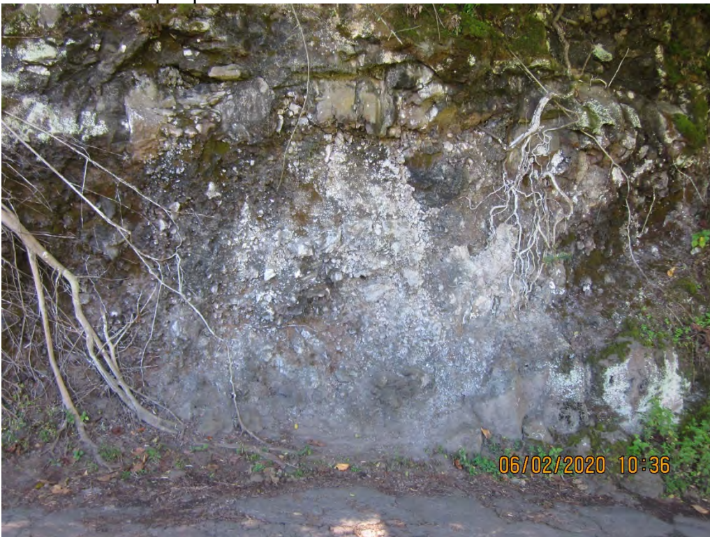
Photo 20. Transect F-W-09, Lower Section. Jointed Basalt with clinker zones and infilling.
