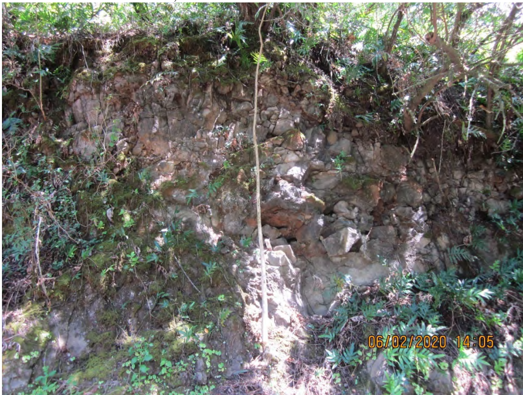
Photo 24. Transect F-W-11, Lower Section. Jointed Basalt with infilling.
