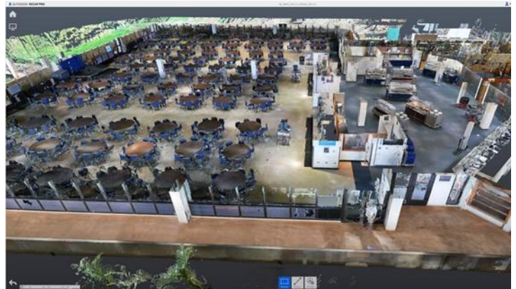
Scans were processed in Autodesk Recap for efficient Revit import
