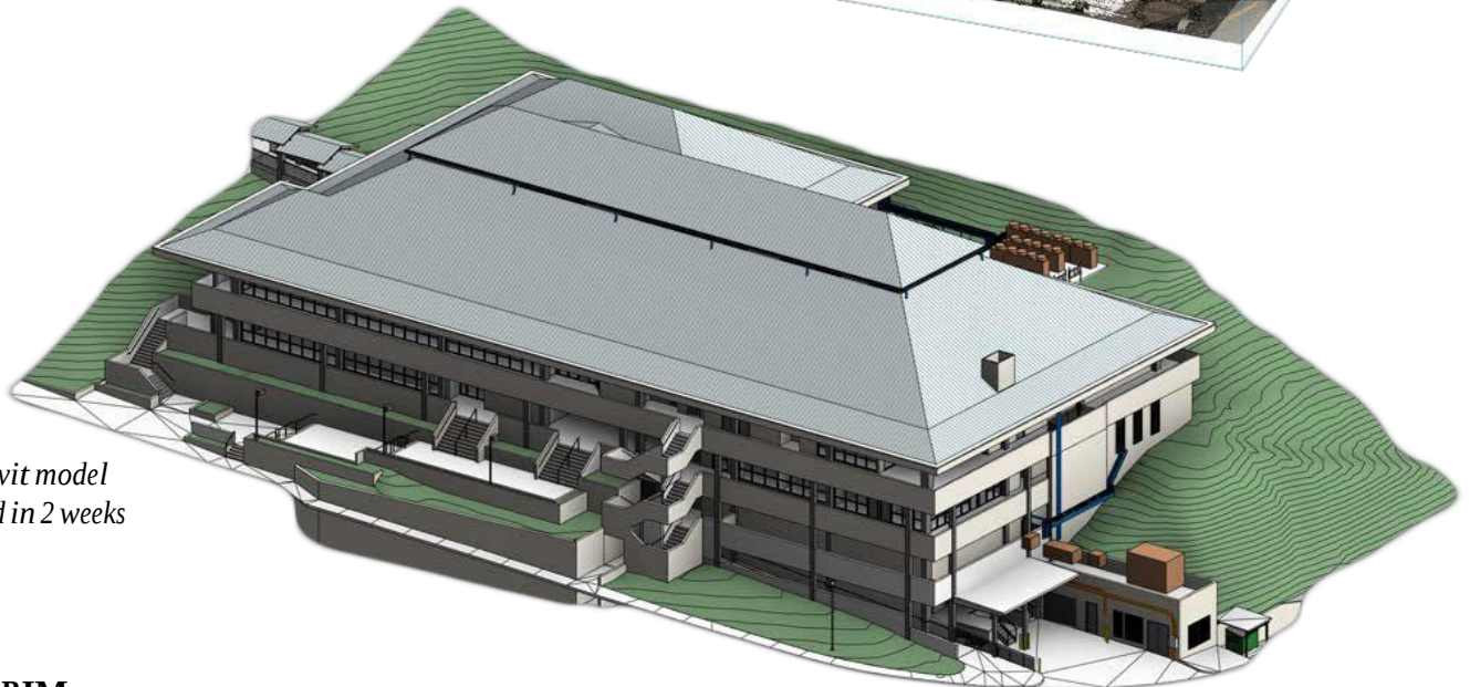
SOH Revit modeling subconsultants created complete Revit model from the laser scans, providing a significant time advantage over Revit modeling from as-built 2D drawings and photographs
