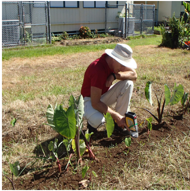
Using XRF, an Integral scientist tests soil in a garden area at a public school.
