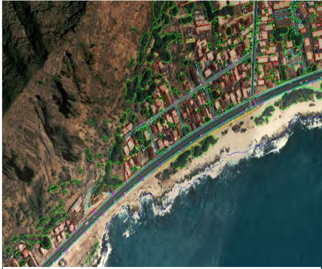
For the 17-mile Farrington Highway Safety Improvements project, RMTC engineers used aerial topographic surveys to support civil design.
