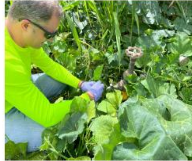
Sampling groundwater from agricultural wells
