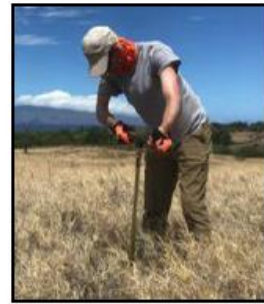
Field personnel using hand auger to obtain incremental samples.
