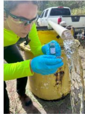
Sampling groundwater from monitoring wells
