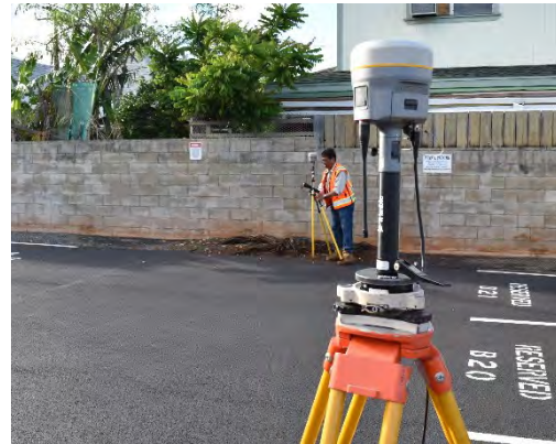
RMTC surveyors conduct field surveys utilizing the latest in GPS technology: the Trimble R10 GNSS System.
