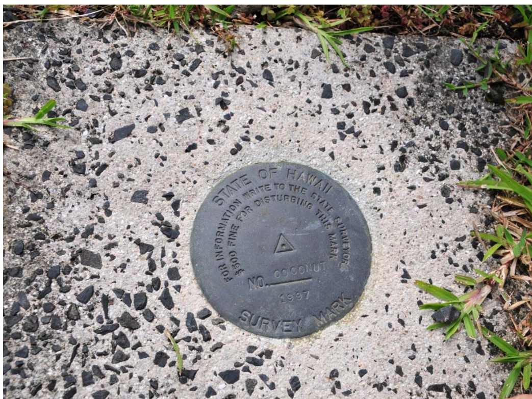
Figure C- 1. Benchmark for GPS Instrument Error Correction.
