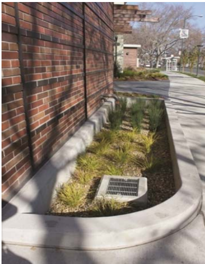
Example of an urban Green Street design using a continuous bioswale planter with drain inlets along the sidewalk and parking lane. (Portland, OR).
