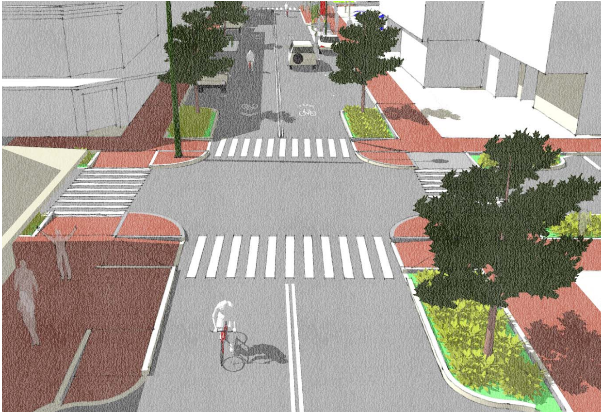
Street trees and bioswale within a curb extension at intersections.
