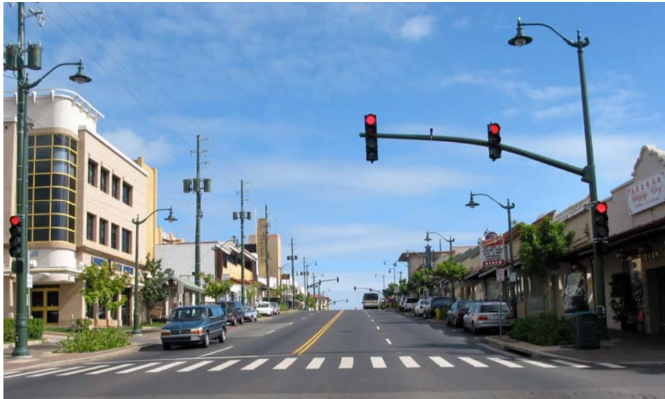
Overhead utilities are maintained on Waiʻalae Avenue in Kaimukī. Tall metal poles were used and power lines oriented vertically for a cleaner look. All vertical streetscape elements were painted dark green.
