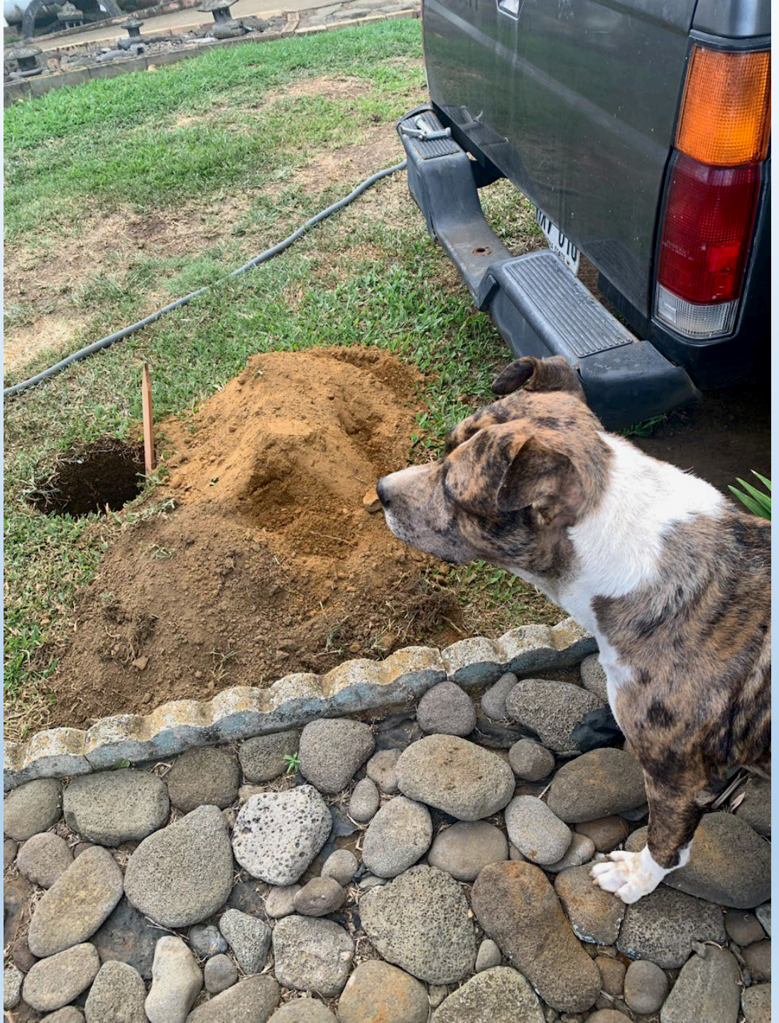
November 2022: Soil percolation testing at four Pāhala homes
