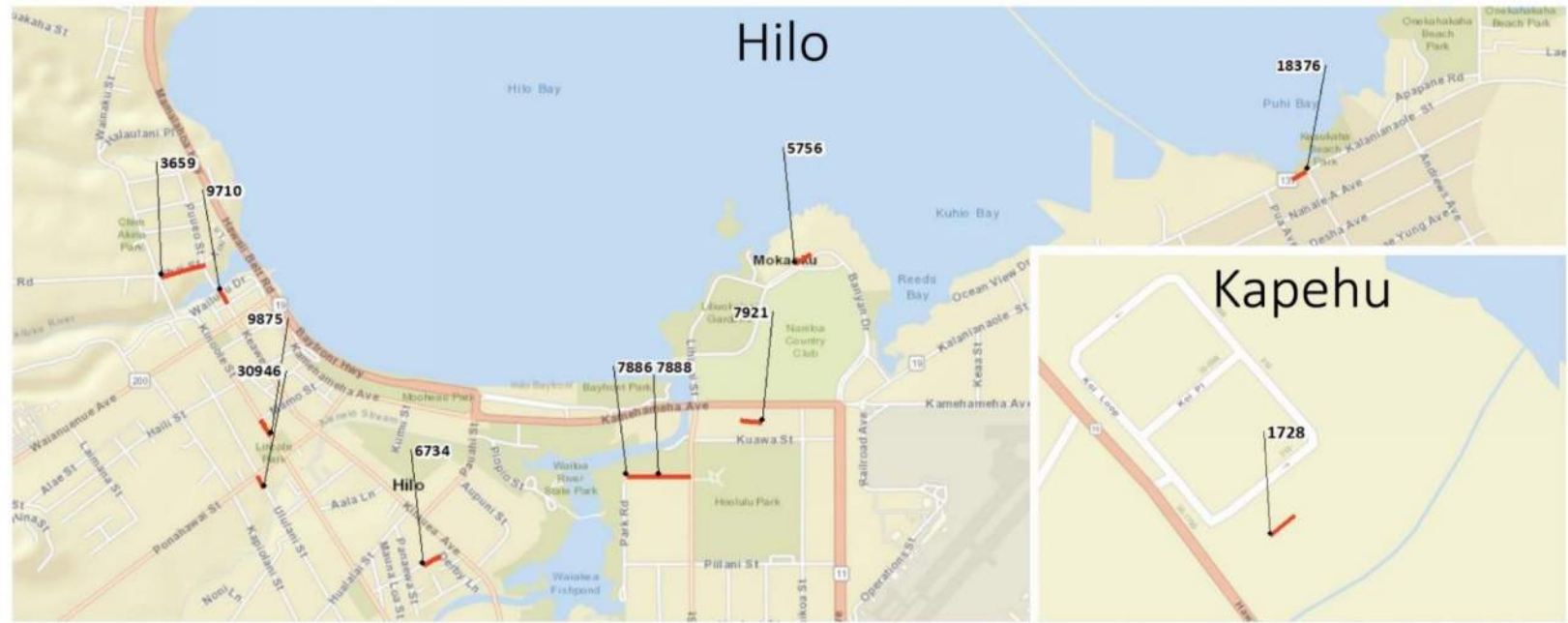
Figure 2: Map of High POF Pipe from CCTV Data
